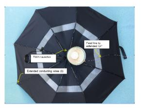
Fig. 2. LP MBWA ensemble in operation for 30-2000 MHz.
