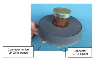
Fig. 3. The TWA Launcher as the prime mover of the LP MBWA ensemble.
